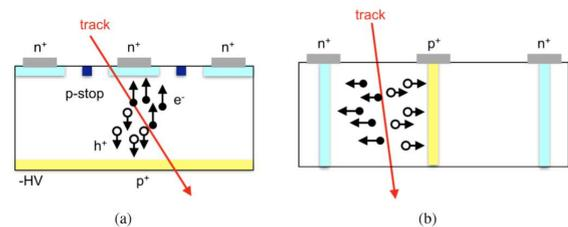
Fig. 1. Description of planar type sensor (a) and 3D type sensor (b)
